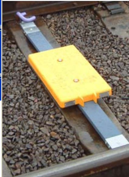
UK e-clip variant with Siemens Balise
